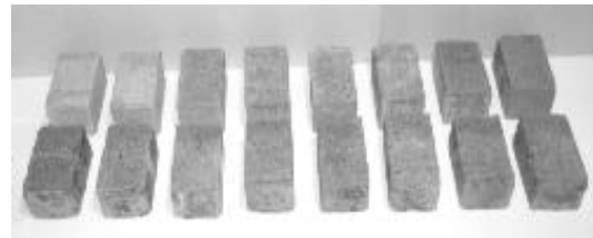
Fig. 2 Split-block samples – after graffiti cleaning
